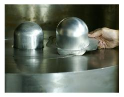
Operating at up to 10,000 psi, this hydroform features and advanced control and hydraulic systems that allows us to precisely manage the forming pressure of punch travel, which facilitates the production of net-shaped parts. Its "open" feature enables our operators to visually inspect parts mid-cycle, after which they can either continue the cycle or abort in order to modify the recipe – a significant time saver in new part development projects.
